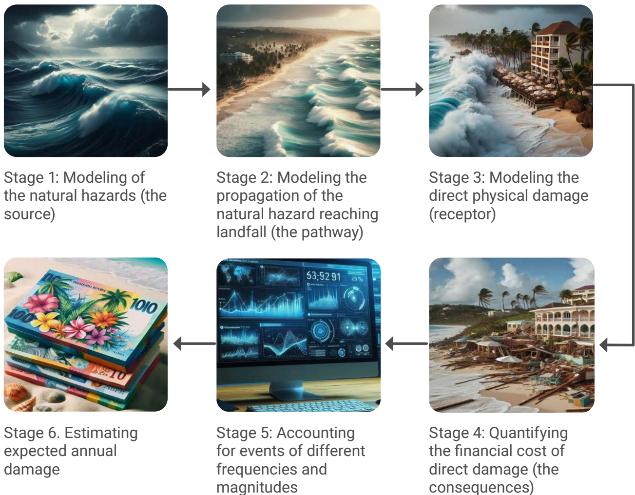
Figure 14. Method used for estimating the expected annual damage (EAD)
