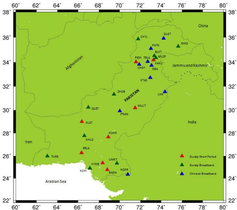
BMD DIGITAL SEISMIC REAL TIME MONITORING NETWORK (EQ INDEX 28)
